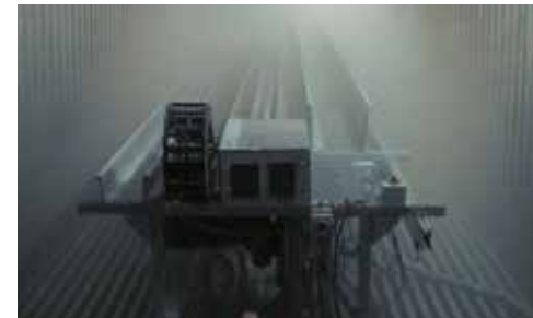
Cold test at -40 °C for chainflex® cables and e-chains®
